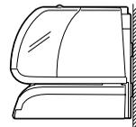
**Note:** Wall mounting should only be performed by authorized Amano dealers. If the PIX-200 is improperly mounted, it could fall, resulting in damage to the unit or personal injury. When mounting the PIX-200 on a concrete wall, or other special wall material, special screws may be required.
