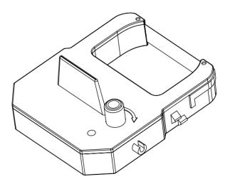
5. Install the ribbon cassette. Position the ribbon is between the print head and the ribbon mask. Printing will not function properly if the ribbon is placed behind the ribbon mask.
