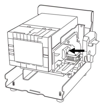
7. Turn the knob of the ribbon cassette in the direction of the arrow to tighten the ribbon.
