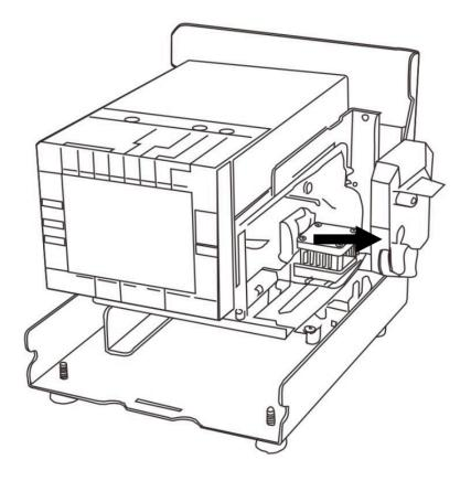
4. Turn the knob of the new ribbon cassette in the direction of the arrow (clockwise) to tighten the ribbon.
