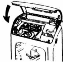
Connect the hooks in the lid (A in the figure) with the hooks in the case (B). Bring the lid down toward you until it is inserted into place.
