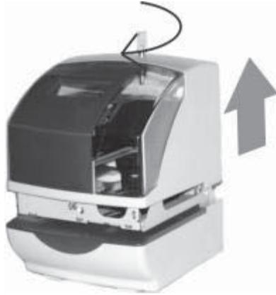
3. Turn the knob of the new cartridge in direction of the arrow (clockwise) to tighten the ribbon.
